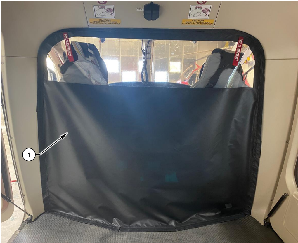
Figure 4 LKG FWD Barrier Assy, (Item 1) Installation Shown.
