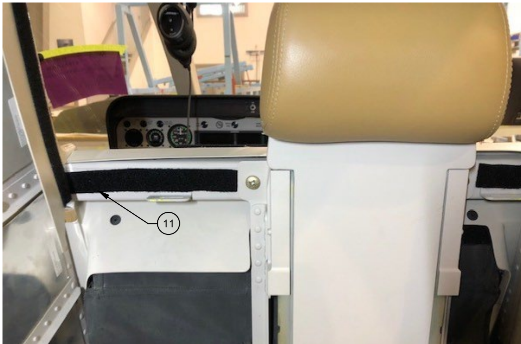
Figure 1 LKG FWD LHS Velcro®, Loop (Item 11) Installation on seatback shown. RHS opposite.
