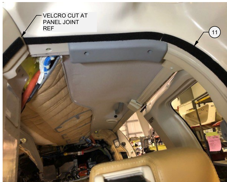
Figure 2 Velcro®, Loop (Item 11) LHS Installation shown. RHS opposite.
